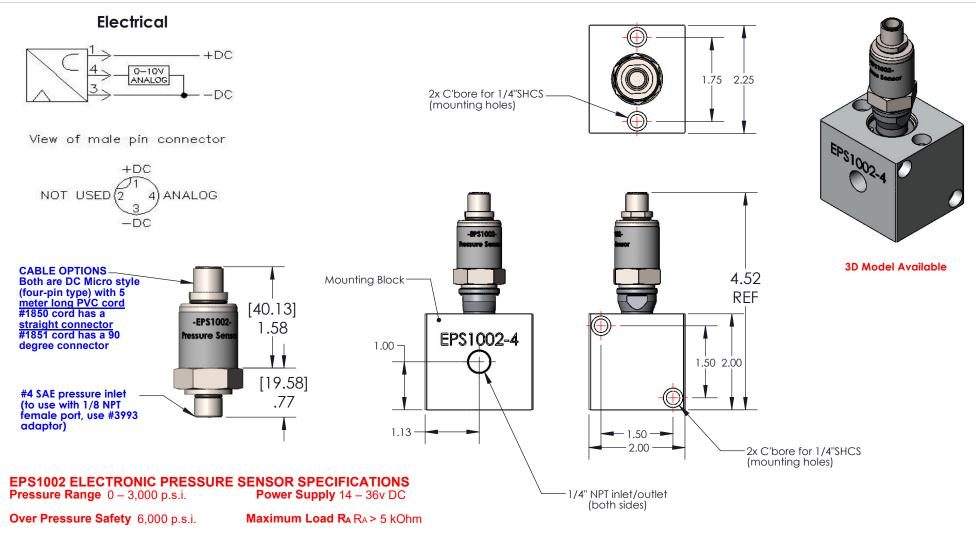
Burst Pressure 7,977 p.s.i. Accuracy (% of span) < 0.4 (BFSL)
