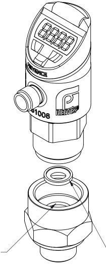
SPECIALTY O-RING SET INCLUDED WITH SENSOR AND MUST BE INSTALLED
