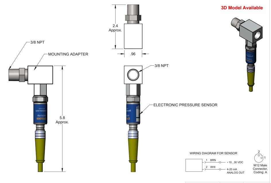
**EPS1009-6**: EPS1009 Assembly with 3/8" NPT mounting adapter.
