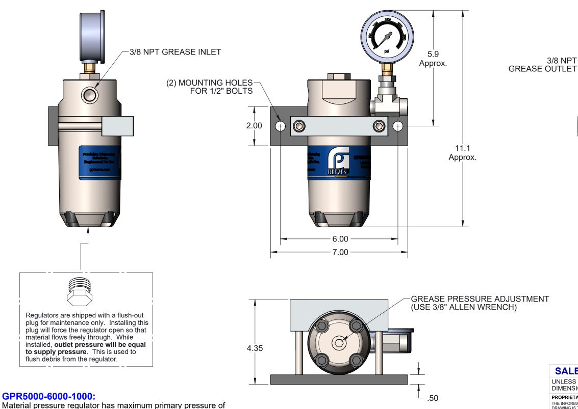
Material pressure regulator has maximum primary pressure of 6,000 psi and controlled secondary pressure between 175 and 1,000 psi. Inlet and outlet ports are 3/8 NPT. Includes mounting bracket for easy panel mounting. Also includes a 0-3,000 PSI output pressure gauge.
